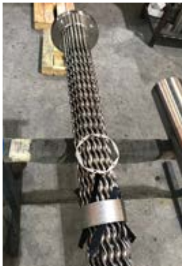
A twisted tube heat exchanger provides better heat transfer and costs less to operate.
