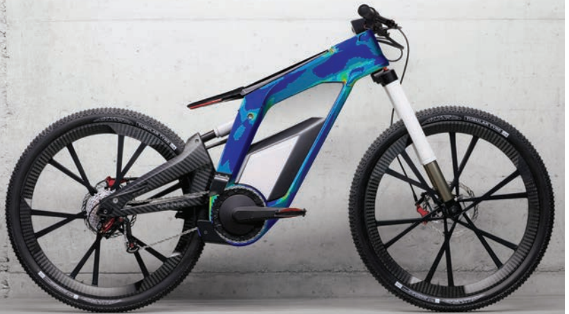
▲ The ultralight carbon frame weighs only 1,600 grams — without sacrificing performance or aesthetic design.
